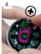
4. Place the new battery on the negative pole and insert it onto the spring.
