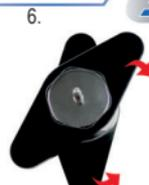
6. Use the opening tool to close the fine thread by turning it clockwise approx. 1/4 turn.
