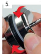
5. Place the loggers on top of each other and first turn the fine thread to the left until the thread can be easily closed by turning it clockwise. Tighten by hand.
