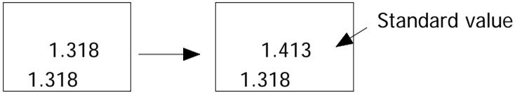
*\* If only intend to make the one point calibration, just execute the 2 mS range ( 1.413 mS Cal. ) is enough.*
